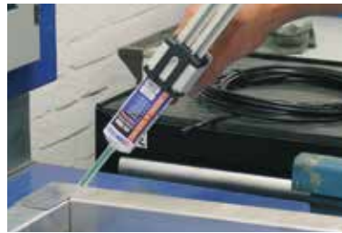
Bonding of aluminium frame
