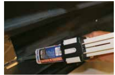
Bonding of metal insert in PP/EPDM bumper
