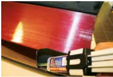
Repair of PP/EPDM bumper
